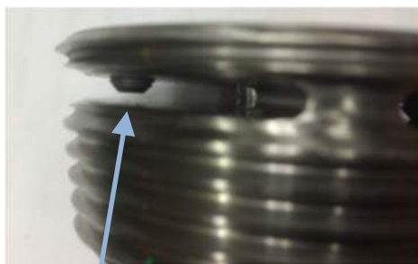
Partially Loose Set screw
