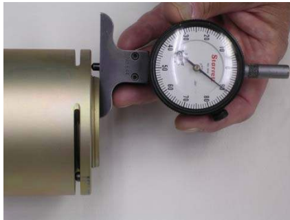
Picture 6H – Use of Drop Gauge to measure stick-out
