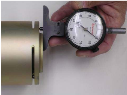
Picture 6J – Use of Drop Gauge to measure stick-out
