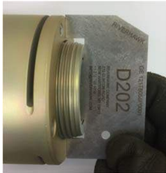
Picture 6H – D202 Gauge to measure stick-out
