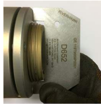
Picture 6G – D652 Gauge to measure stick-out
