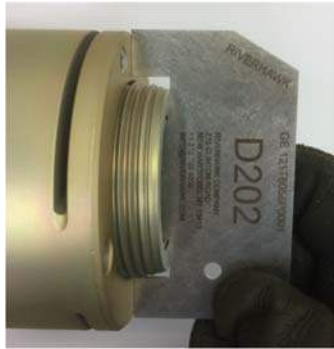
Picture 6H – D202 Gauge to measure stick-out
