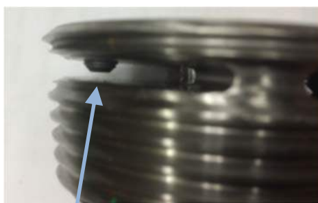
Partially Loose Set screw
