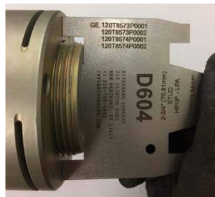
Picture 6E – Use of D604 Stick-Out Gauge on LPA-LPB Flange
