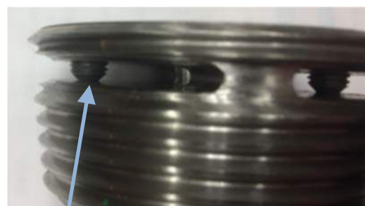
Pressed against Opposite Surface. No Gap.
