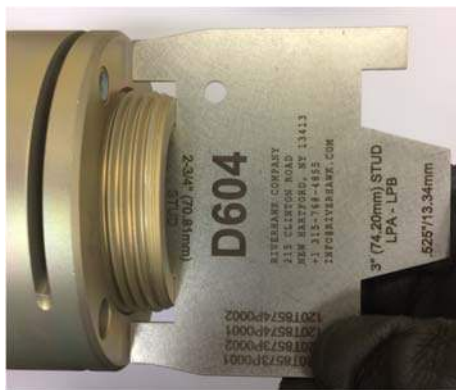
Picture 6D – Use of D604 Stick-Out Gauge on HP/IP-LPA Flange
