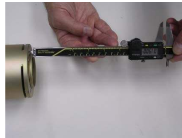
Picture 6F – Use of Calipers to measure stick-out
