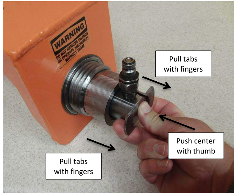
Picture 11B - Activation of the safety interlock
