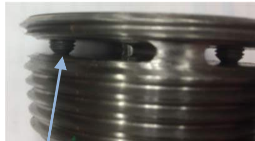
Pressed against Opposite Surface. No Gap.
