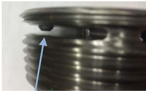
Partially Loose Set screw
