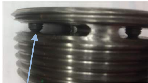
Pressed against Opposite Surface. No Gap.
