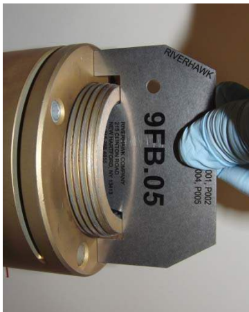
Picture 6C – Use of Stick-Out Gage on the Gas Turbine side of the Flange Joint
