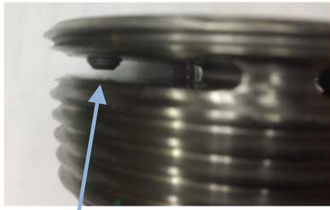
Partially Loose Set screw
