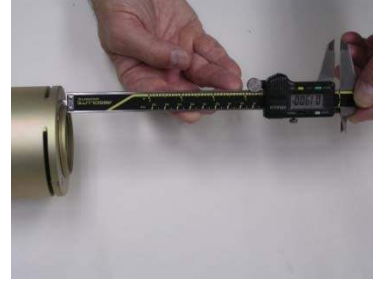
Picture 6F – Use of Calipers to measure stick-out
