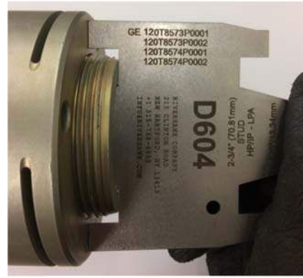
Picture 6E – Use of D604 Stick-Out Gage on LPA-LPB Flange
