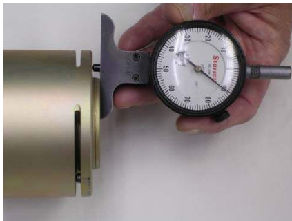
Picture 6G – Use of Drop Gage to measure stick-out
