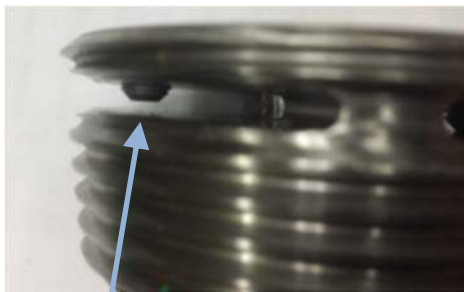
Partially Loose Set screw
