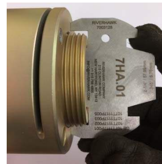
Picture 6D – Use of Stick-Out Gage on the Generator side of the Load Coupling
