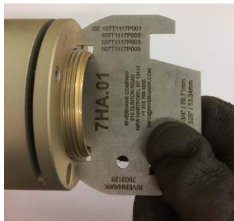
Picture 6C – Use of Stick-Out Gage on the Gas Turbine side of the Load Coupling (Gage appearance may vary)
