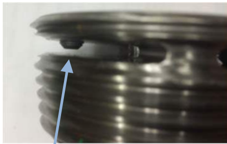
Partially Loose Set screw
