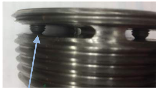
Pressed against Opposite Surface. No Gap.
