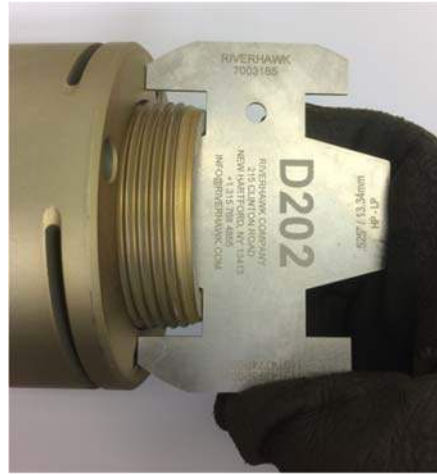
Picture 6F – Use of a D202 Stick-Out Gage on a LP/GENERATOR flange.
