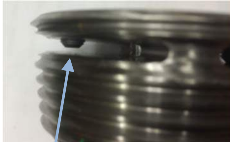
Partially Loose Set screw
