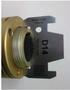
Picture 6E – D14 Gage to measure stick-out
