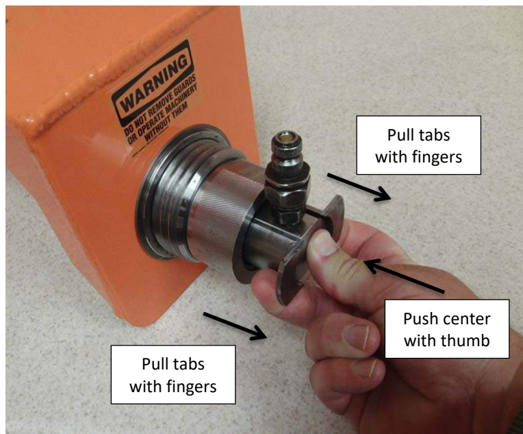
Picture 8C - Activation of the safety interlock
