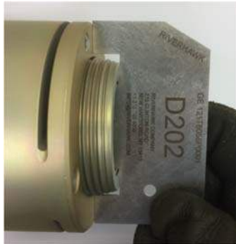
Picture 6G – D202 Gage to measure stick-out
