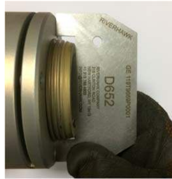
Picture 6F – D652 Gage to measure stick-out
