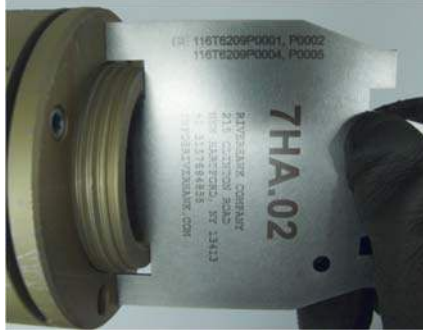
Picture 6G – Use of Stick-Out Gage on the 3” Stud
