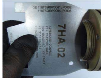
Picture 6H – Use of Stick-Out Gage on the 2-1/4” Stud
