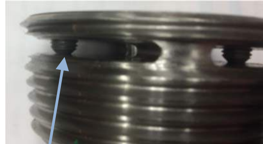
Pressed against Opposite Surface. No Gap.
