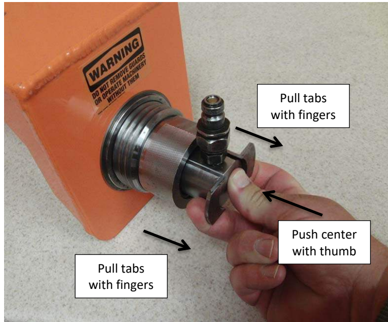
Picture 8C - Activation of the safety interlock
