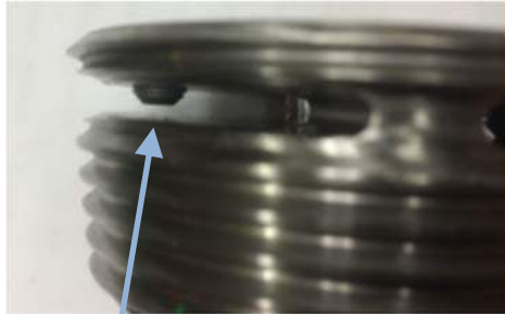
Partially Loose Set screw
