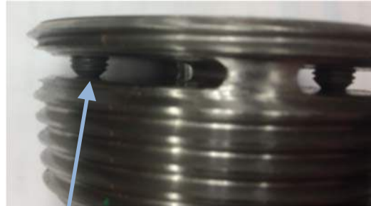
Pressed against Opposite Surface. No Gap.
