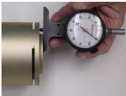
Picture 6F – Use of Drop Gage to measure stick-out
