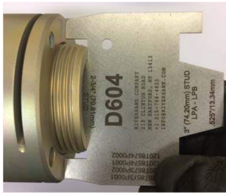
Picture 6D – Use of D604 Stick-Out Gage on HP/IP-LPA Flange
