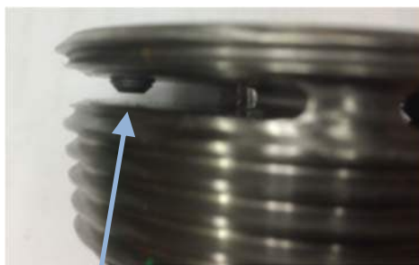
Partially Loose Set screw
