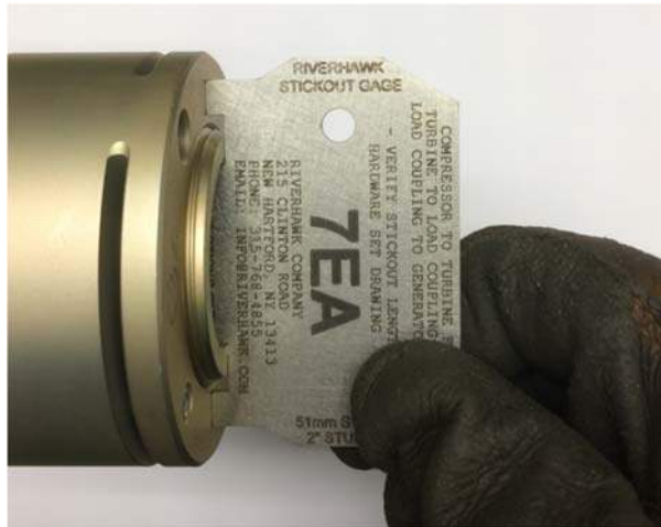
Picture 6D – Use of Stick-out Gage
