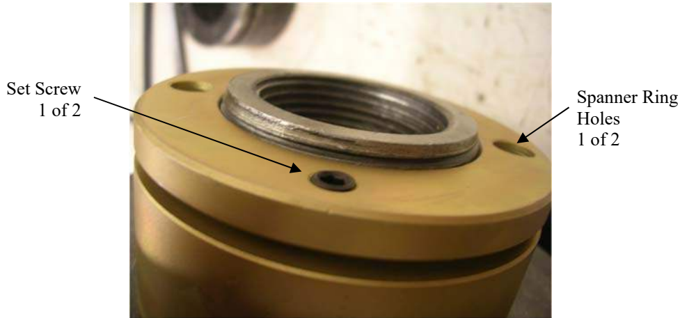
Picture 10A – Riverhawk Locknut
