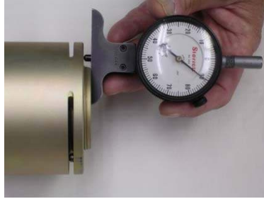
Picture 6E – Use of Drop Gage to measure stick-out
