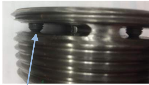
Pressed against Opposite Surface. No Gap.
