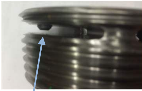
Partially Loose Set screw
