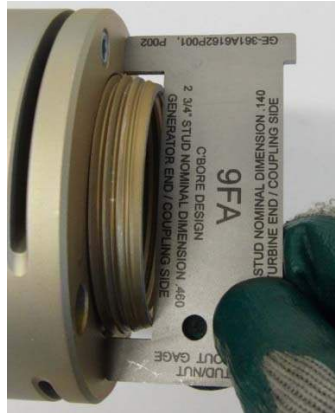
Picture 6D – Use of Stick-Out Gage on Load Coupling to Generator Bolted Flange Connection
