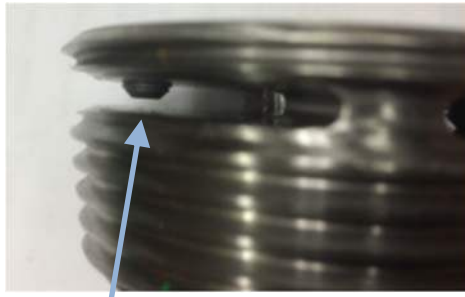
Partially Loose Set screw
