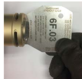
Picture 6D – Use of Stick-Out Gage on the 6F.03 Load Coupling stud
