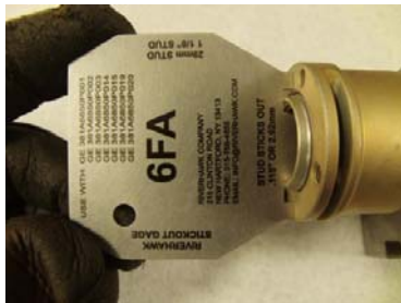
Picture 6C – Use of Stick-Out Gage on the 6FA Load Coupling stud
