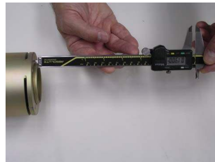
Picture 6K – Use of Calipers to measure stick-out
