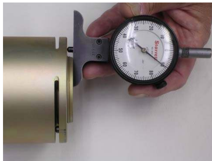
Picture 6J – Use of Drop Gage to measure stick-out
