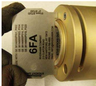
Picture 6D – Use of Stick-Out Gage on the 6FA Generator stud
