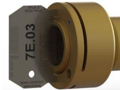
Figure 6H – Use of Stick-Out Gage on the 7E.03 stud
