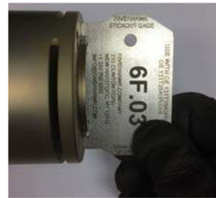
Picture 6E – Use of Stick-Out Gage on the 6F.03 Generator stud
