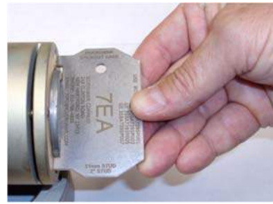
Picture 6G – Use of Stick-Out Gage on the 7E or 7EA stud
