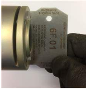
Picture 6F – Use of Stick-Out Gage on the 6F.01 Generator stud
