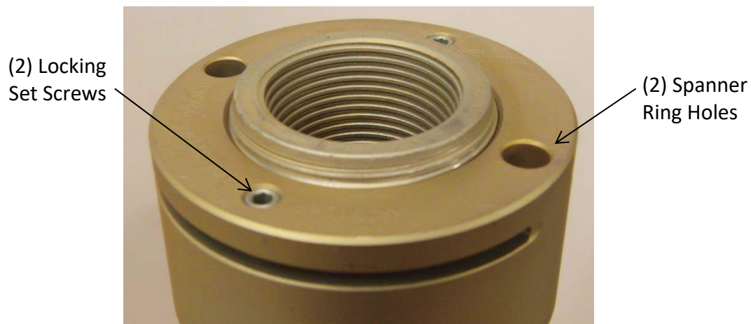
Picture 5A - Riverhawk Locknut
