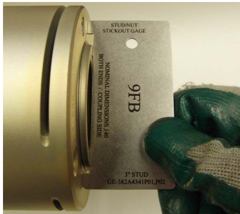
Picture 6C – Use of Stick-Out Gage
