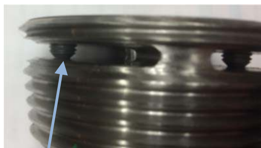
Pressed against Opposite Surface. No Gap
