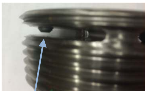
Partially Loose Set screw
