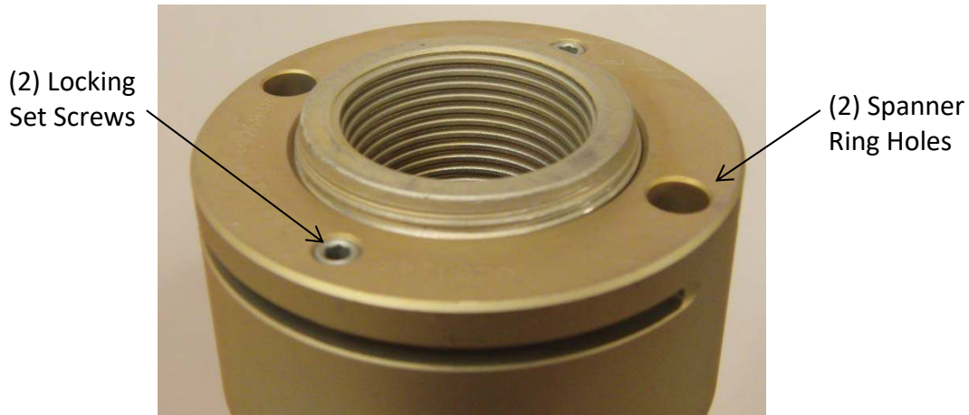
Picture 10A - Riverhawk Locknut
