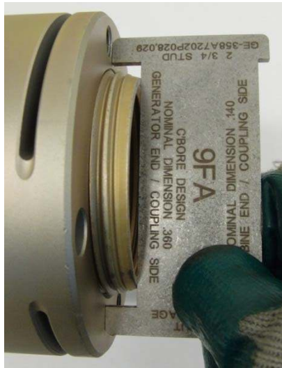
Picture 3 – Use of Stick-Out Gage on Load Coupling or Steam Turbine to Generator Counterbored Flange Connection
