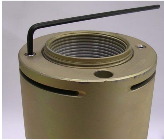
Picture 6 - Loosening of a nut's set screws
