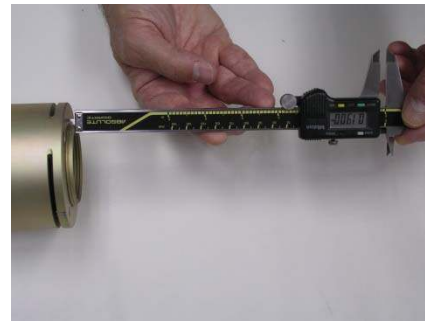
Picture 6D – Use of Calipers to measure stick-out
