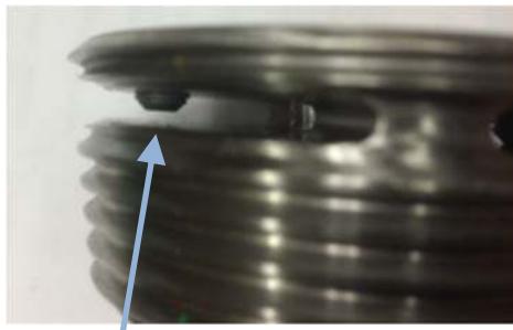
Partially Loose Set screw
