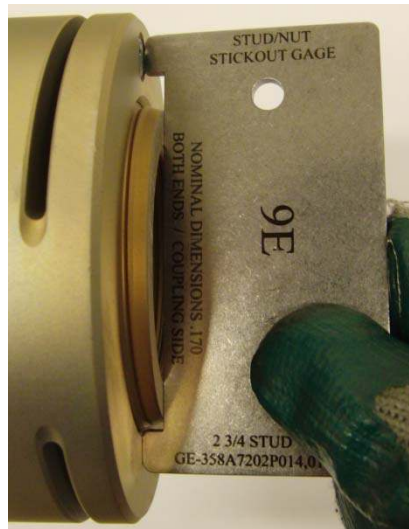
Picture 6E – Use of Stick-Out Gage (Stick-out gage appearance may vary)
