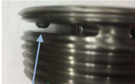
Partially Loose Set screw
