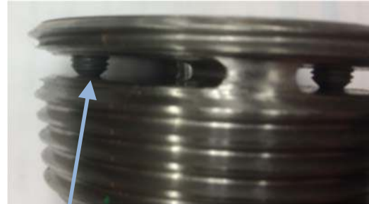
Pressed against Opposite Surface. No Gap.
