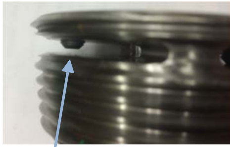
Partially Loose Set screw
