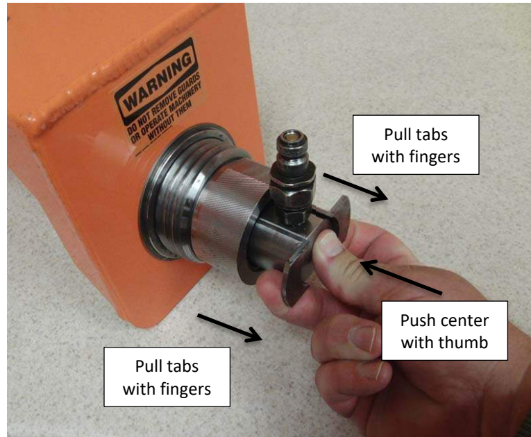
Picture 11B - Activation of the safety interlock
