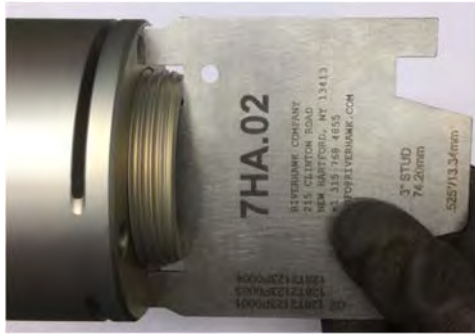
Picture 6J – Use of Stick-Out Gage on the 2-3/4" Stud
