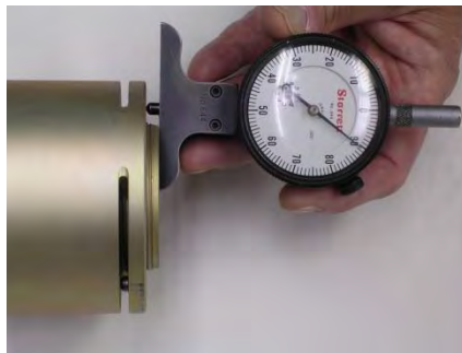
Picture 6N – Use of Drop Gage to measure stick-out
