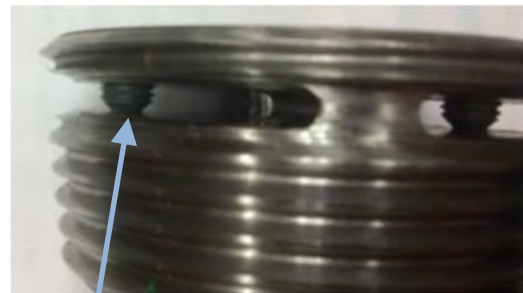
Pressed against Opposite Surface. No Gap.
