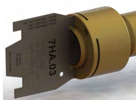
Figure 6M – Use of Stick-Out Gage on the 2-1/4" Stud
