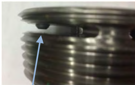
Partially Loose Set screw
