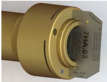
Figure 6L – Use of Stick-Out Gage on the 3" Stud
