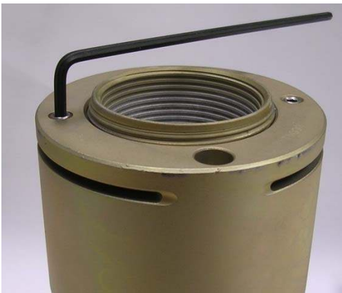
Picture 6 - Loosening of a nut's set screws
