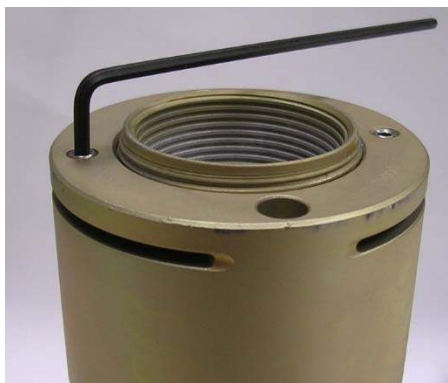
Picture 6 - Loosening of a nut's set screws
