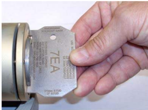
Picture 6D – Use of Stick-out Gage
