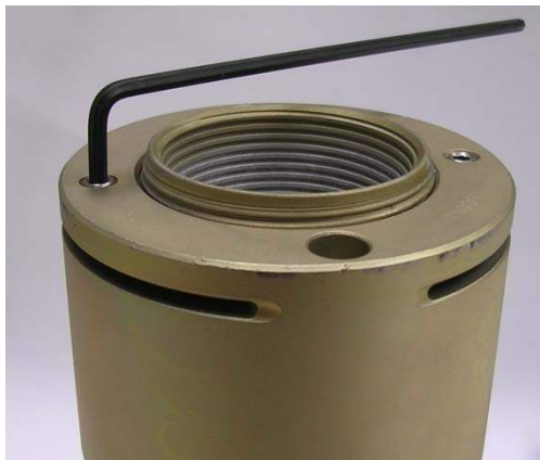
Picture 6 - Loosening of a nut's set screws
