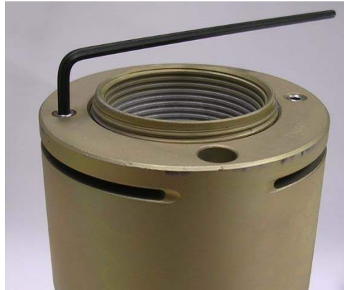
Picture 11B - Loosening of a nut's set screws
