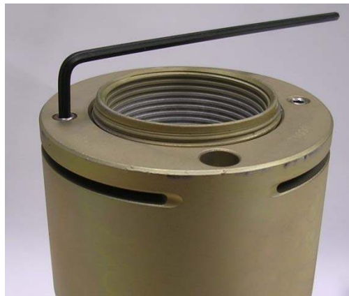
Picture 6 - Loosening of a nut's set screws
