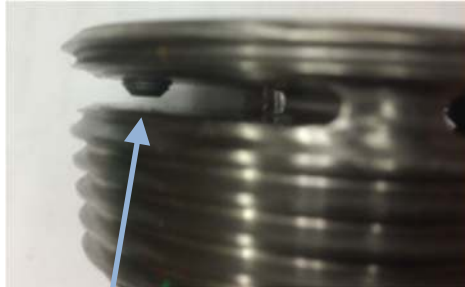
Partially Loose Set screw
