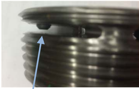
Partially Loose Set screw
