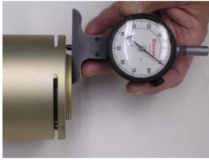
Picture 6H – Use of Drop Gage to measure stick-out
