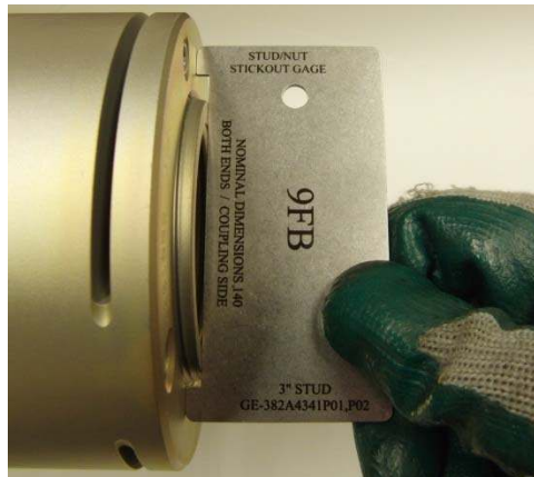
Picture 6C – Use of Stick-Out Gage
