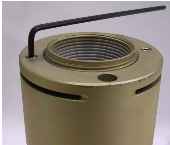
Figure 11D - Loosening of a nut's set screws
