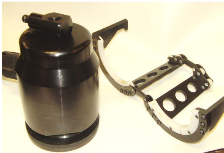
Figure 8A – Hydraulic cylinder and lifting cradle
