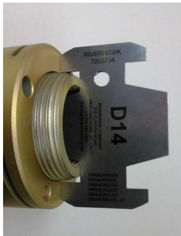
Figure 6A – Use of gage to measure stick-out
