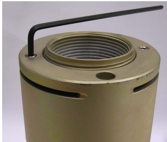
Picture 6 - Loosening of a nut's set screws
