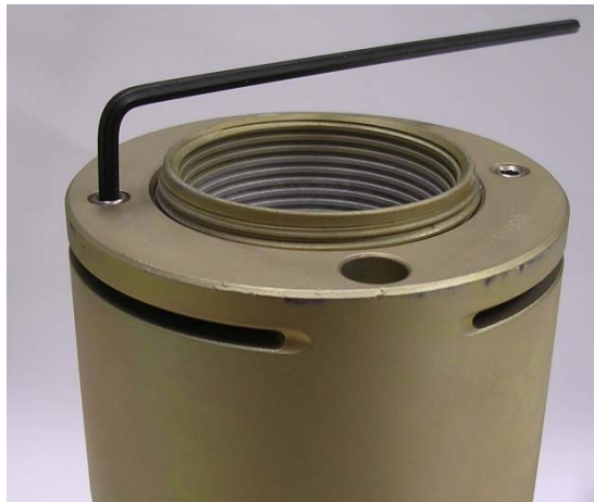
Sample Picture of the loosening of a nut's set screws
