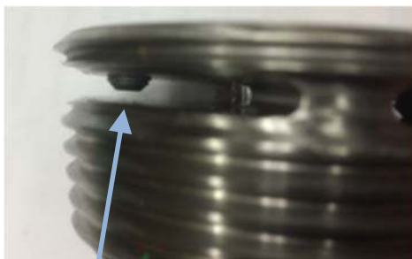
Partially Loose Set screw
